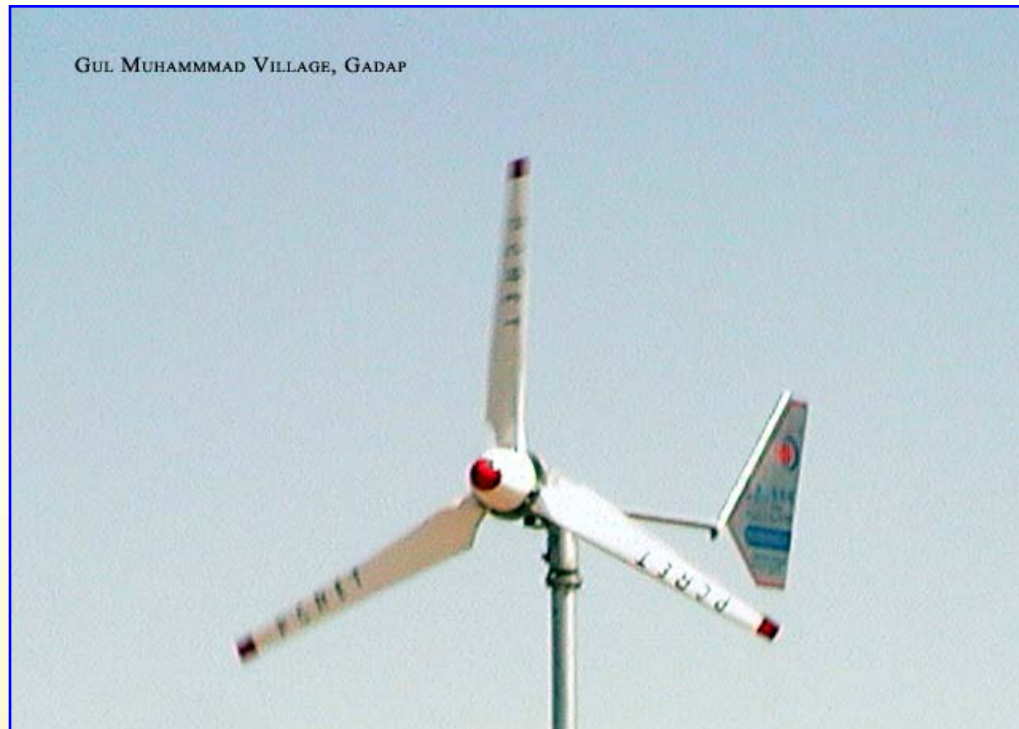
Wind turbine (5 KW) for power supply to house holds at Kemari Town Karachi
